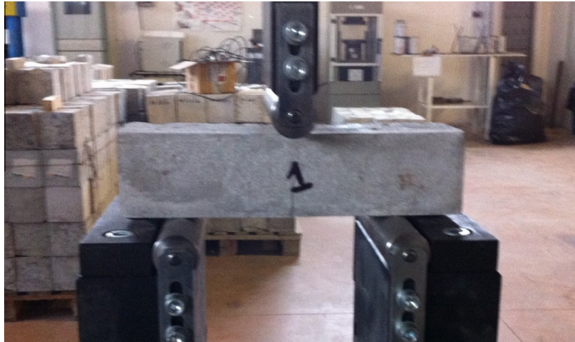
Fig. 5. Three-point bending test setup.
