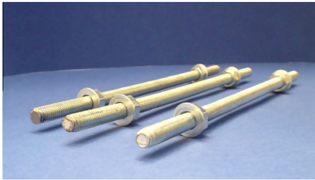
Fig. 9. Photograph of the bars prepared for the insertion of the string network.
