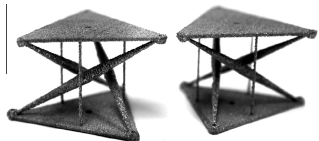
Fig. 3. EBM-printed left-handed (left) and right-handed (right) tensegrity prisms.
