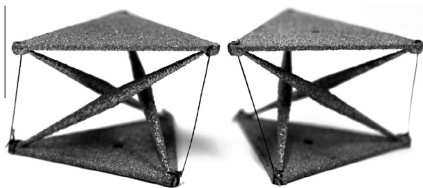
Fig. 6. L-prism (left) and R-prism (right) samples obtained by 'sewing' the EBM-printed models with Spectra strings.
