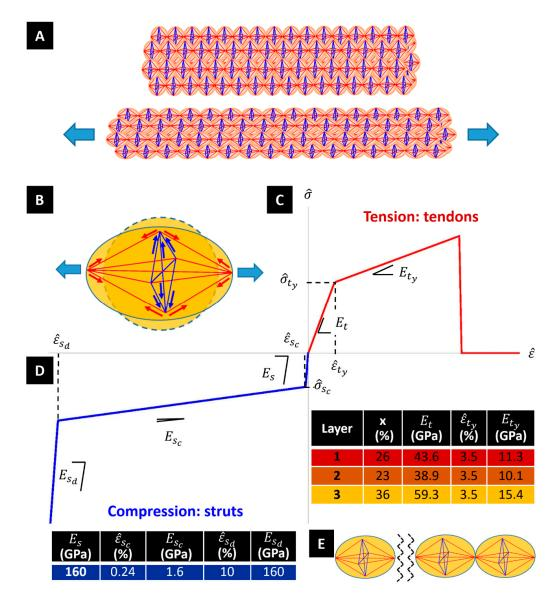
**Figure 2.** (**A**) Bundle of tensegrity fibrils (red members are tendons, while blue members are struts) and deformation mechanism under tensile loading. (**B**) The tendons are loaded in tension, while the struts are loaded in compression. Stress-strain responses of struts (**C**) and tendons (**D**) alongside their respective mechanical parameters. (**E**) Fracture of a fibril at the interface between two adjacent units.
