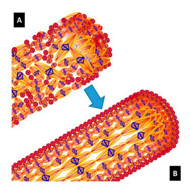
**Figure 6.** Design of artificial fibres with graded tensegrity architecture (**B**) may enable higher performance space to be accessed, as well as a graded crystalline nanostructure of the fibrils, compared to random structure (**A**).
