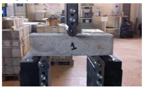
Figure 5 – Three-point bending test setup.
