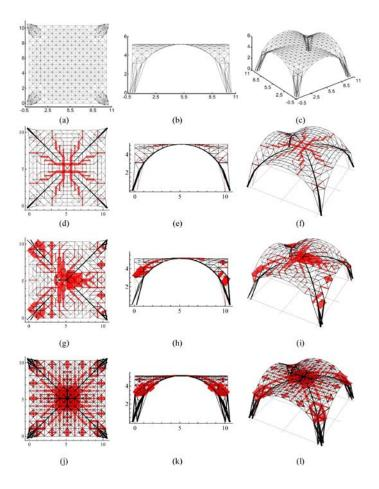
Figure 4: Top, side and 3D views of the optimal reinforcement patterns of a groin vault with FRP/FRCM strips of thickness 0.17 mm on the web panels, and 200 mm  $\times$  3.24 mm FRCM strips or 11.18 mm radius pultruded FRP profiles at the corners (reinforcements marked in red). (a)-(c): Background structure. (d)-(f): Vertical loading. (g)-(i): Seismic loading in the +*x*-direction. (j)-(l): Combined vertical loading and seismic loading in two perpendicular directions.
