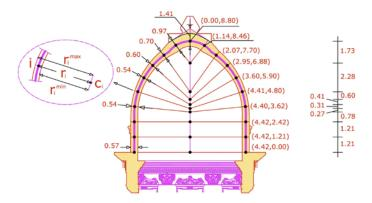
Figure 2: Cross-section of the dome of the church of Santa Maria di Monteverginella in Naples.
