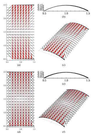
Figure 6: Top, side and 3D views of the optimal reinforcement patterns of a barrel vault with FRP/FRCM strips of thickness 0.17 mm (marked in red). The widths of the FRP/FRCM reinforcements are magnified by a factor 10 for visual clarity. (a)-(c): Seismic loading in the +x-direction. (d)-(f): Combined vertical loading and seismic loading in two perpendicular directions.
