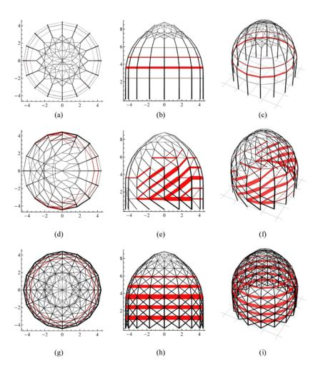
Figure 3: Top, side and 3D views of the optimal reinforcement patterns of a masonry dome with FRP/FRCM strips of thickness 0.34 mm (marked in red), under different loading conditions. (a)-(c): Vertical loading. (d)-(f): Seismic loading in the +x-direction. (g)-(i): Combined vertical loading and seismic loading in two perpendicular directions.
