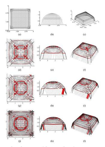
Figure 5: Top, side and 3D views of the optimal reinforcement patterns of a cloister vault with FRP/FRCM strips of thickness 0.17 mm (marked in red), under different loading conditions. The widths of the FRP/FRCM reinforcements are magnified by a factor 2 for visual clarity. (a)-(c): Background structure. (d)-(f): Vertical loading. (g)-(i): Seismic loading in the +*x*-direction. (j)-(l): Combined vertical loading and seismic loading in two perpendicular directions.
