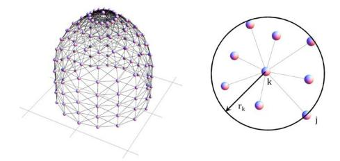
Figure 1: Background structure associated with a node set extracted from a dome (left) and nearest neighbors of a selected node (right).
