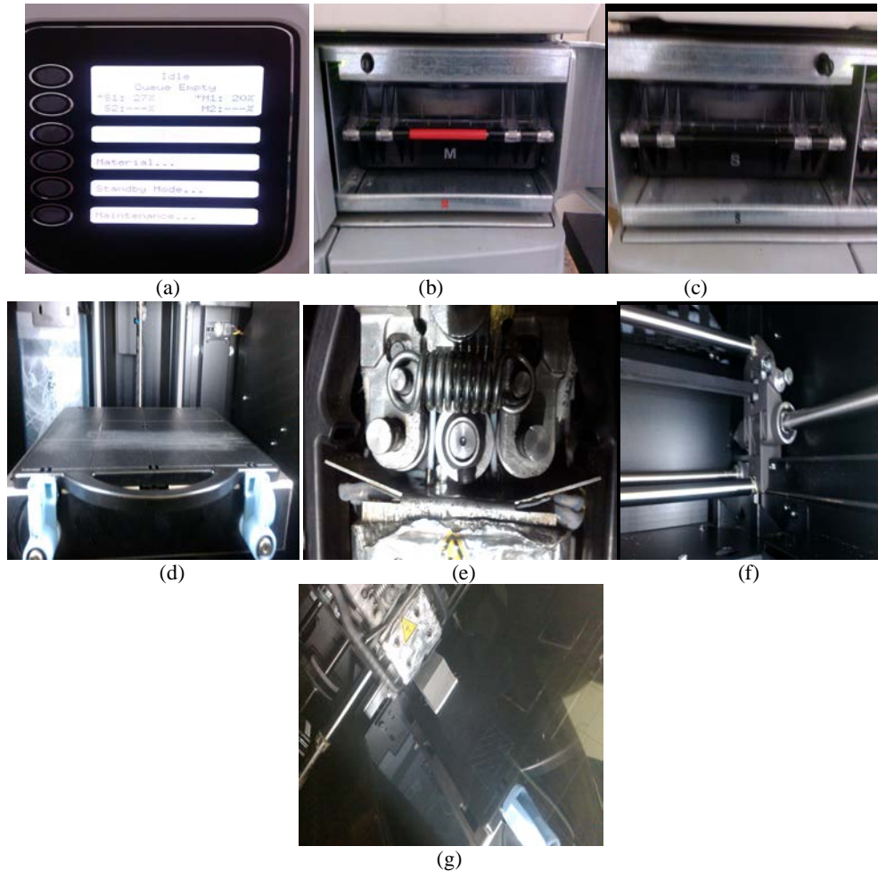
Note: (a) Controlling display; (b) Model material rack; (c) Support material rack; (d) Base platform; (e) Roller screw; (f) Mechanical drives; (g) Building prototypes
