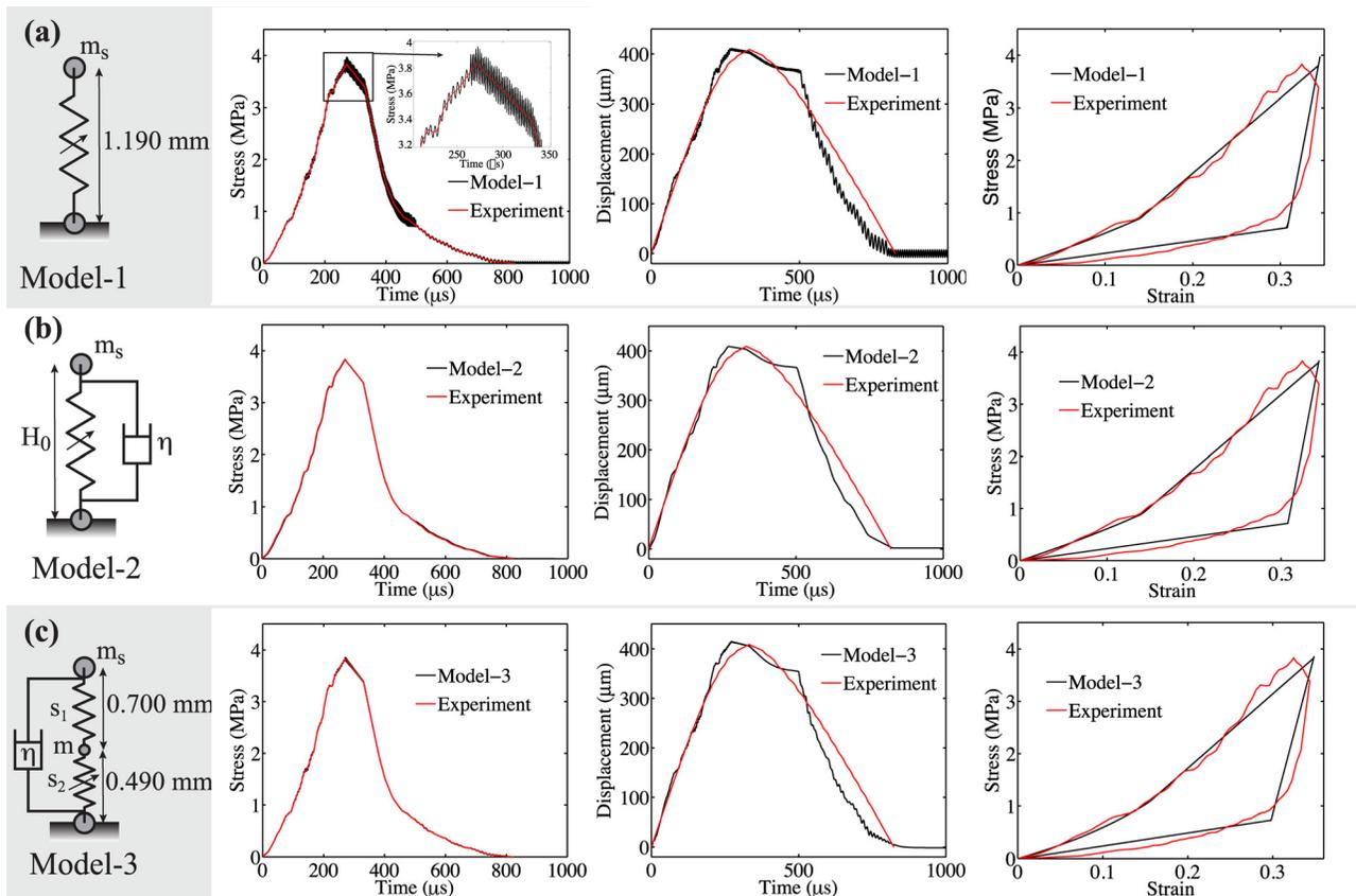
**Fig. 3 Comparison of the numerical and experimental results of stress–time histories, displacement–time histories, and stress–strain response for (a) model-1, (b) model-2, and (c) model-3 of the VACNT foam-1**
