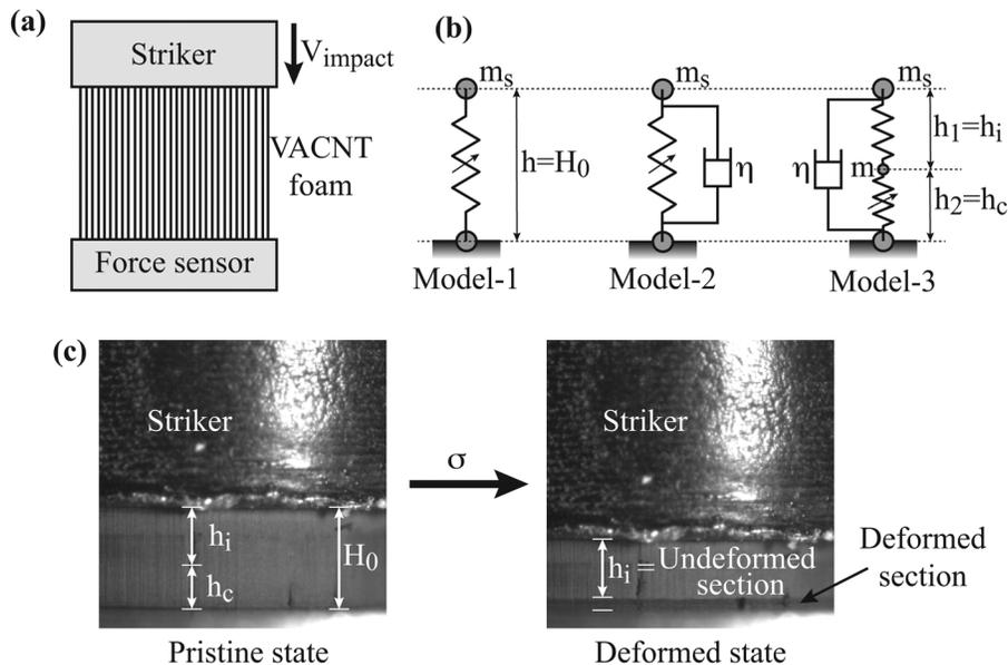
**Fig. 2** Description of the model for the sample impacted at  $1.75 \text{ ms}^{-1}$ . (a) Schematic of the experiment showing the sample being compressed by the striker against the rigidly mounted force sensor. (b) Three different models considered for the sample. (c) Optical images showing the pristine and deformed states of the sample [7]. Markers are used to highlight the deformed and undeformed sections of the sample.
