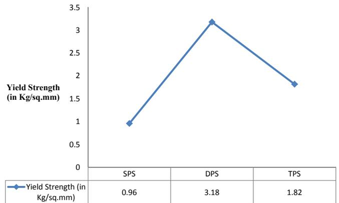
Fig. 9. Plot for yield strength with change in particle size.
