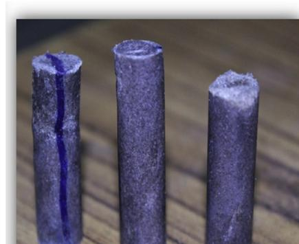
Fig. 6. Manufactured pins on FDM.
