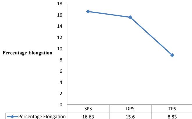
Fig. 7. Plot for percentage elongation with change in particle size.
