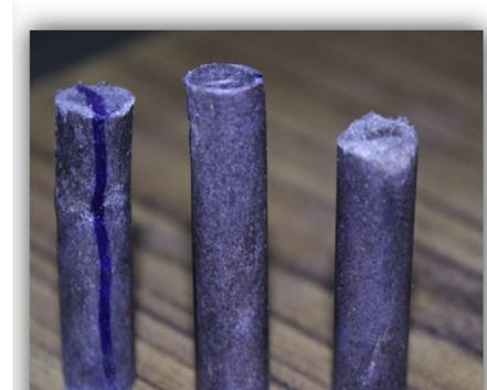
**Fig. 6.** Manufactured pins on FDM.
