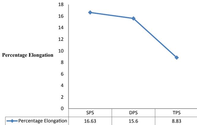
Fig. 7. Plot for percentage elongation with change in particle size.
