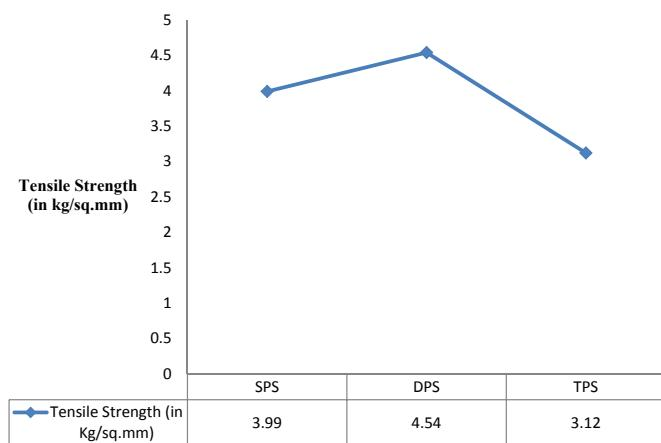
Fig. 8. Plot for tensile strength with change in particle size.
