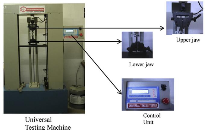
Fig. 3. 3D view of UTM and its parts.
