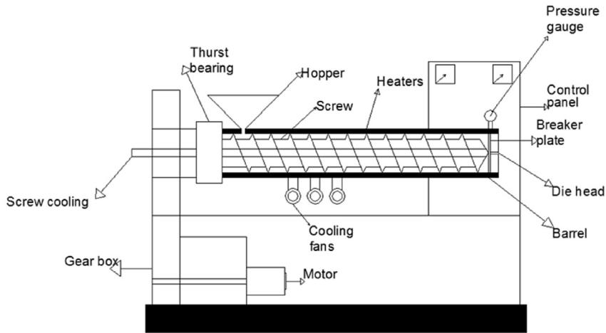
**Fig. 4.** Schematic of single screw extruder machine [15].
