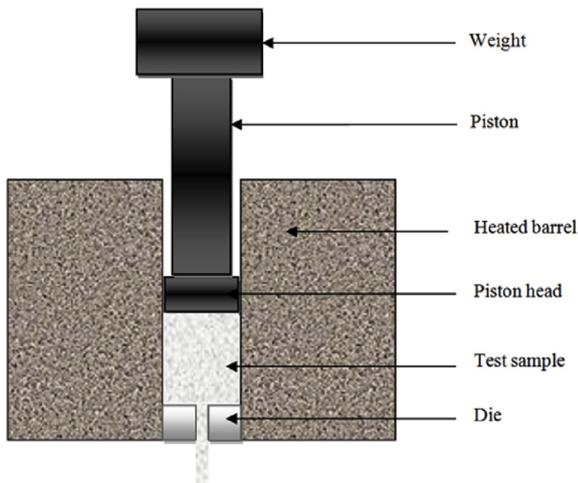
Fig. 2. Schematic of MFI tester [14].
