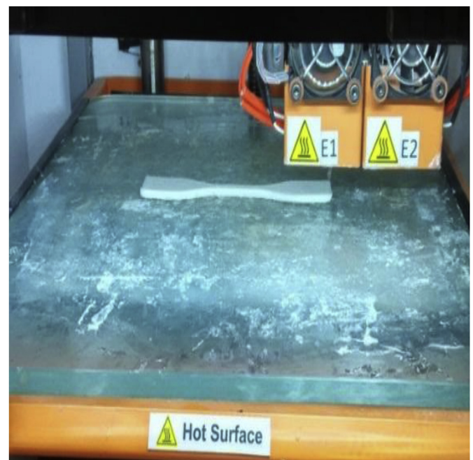
Fig. 3. FDM setup used for 3D printing.
