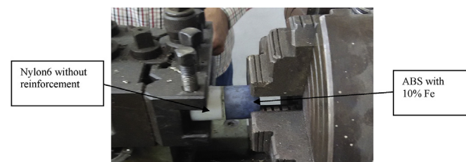
Fig. 1. Pilot experimentation on Center lathe.
