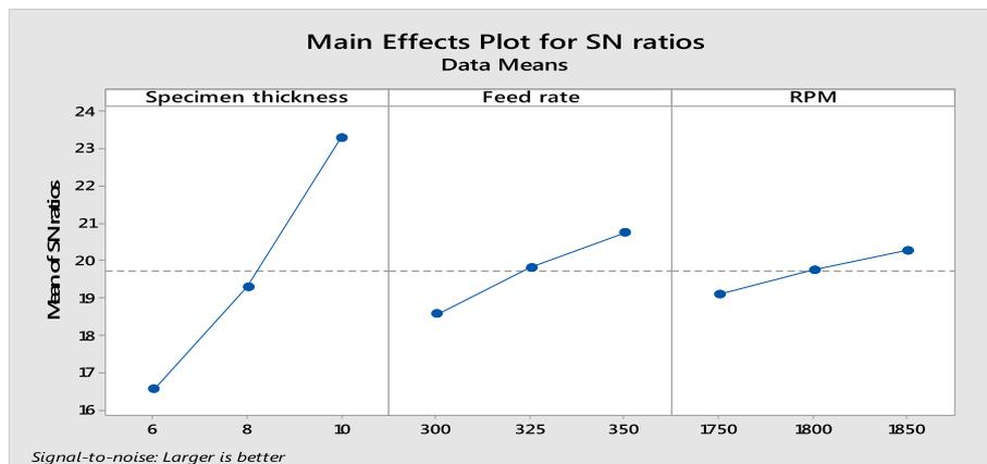
Fig. 3. Main effects plot for SN ratios of tensile strength.
