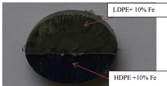
Fig. 1. Pilot experimentation of LDPE and HDPE friction stir welding.
