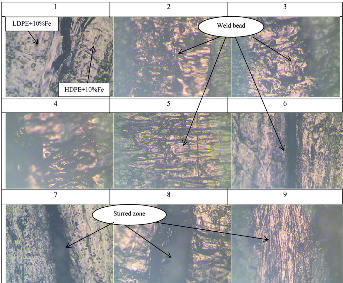
Fig. 5. Optical micrographs for reinforced Fe powder joints (at magnification of 100x).
