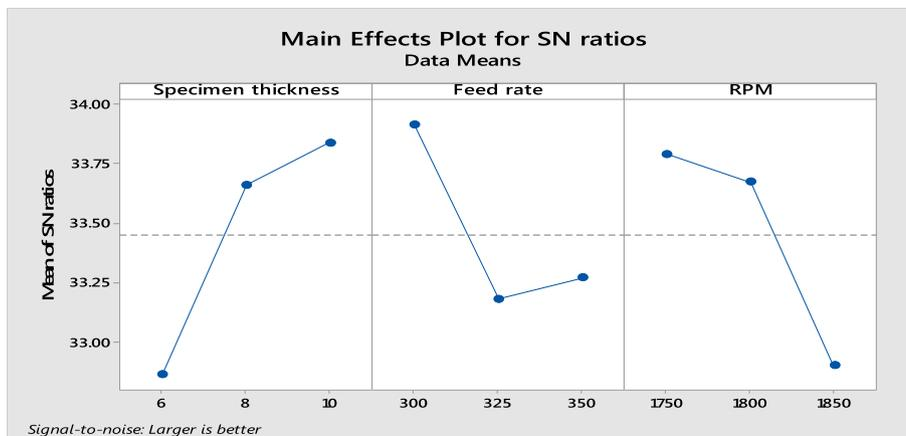
Fig. 2. Main effects plot for SN ratios of shore D hardness.
