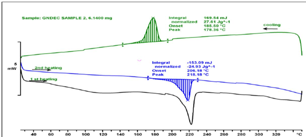
Fig. 3. DSC thermograms for NC.
