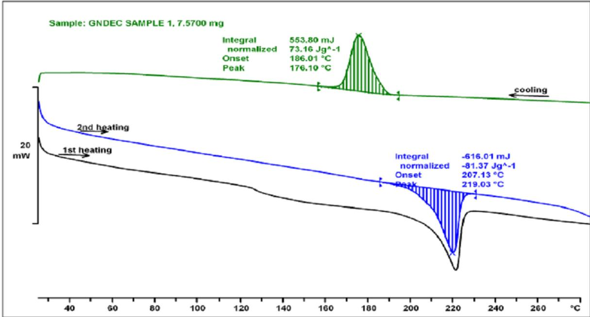
Fig. 2. DSC thermograms for waste Nylon6.
