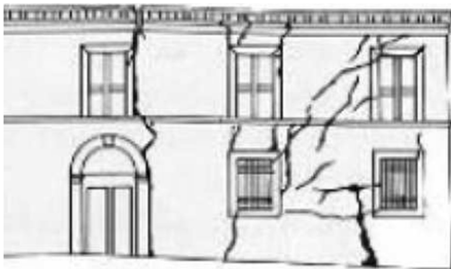
Fig. 2 The façade of a XVII century building exhibiting a manifest crack pattern due to a foundation settlement (courtesy of Prof. Paolo Faccio, IUAV Venezia)
