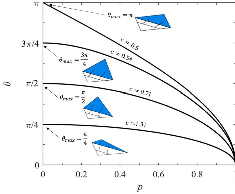
Fig. 13. Opening angle  $\theta$  as a function of the base coordinate  $p$ , for  $a = 1$  and different values of  $c$ . The insets show the configuration of the micro-triangle in the fully open placement ( $\theta = \theta_{max}$ ).
