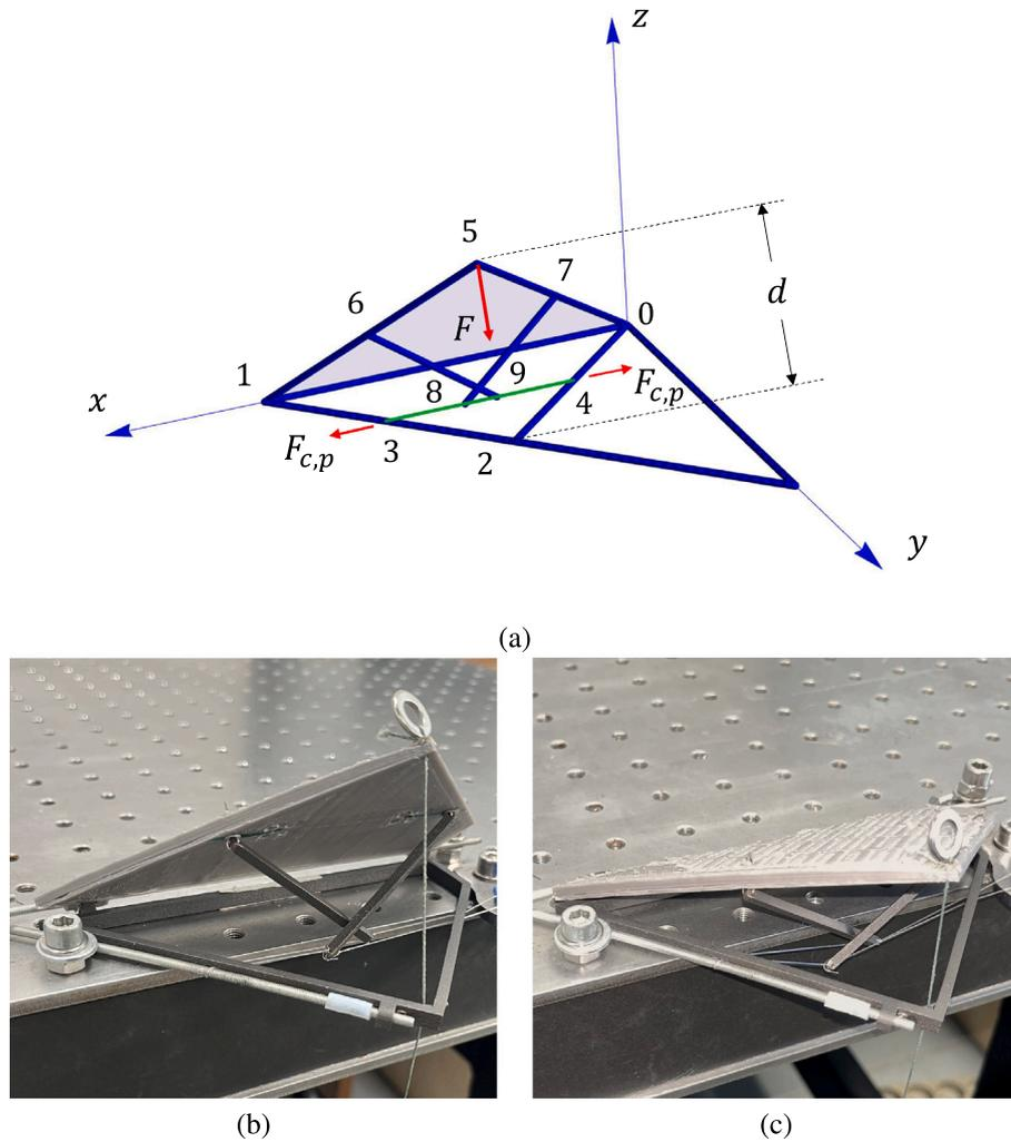
**Fig. 18.** Illustration of the mechanical and physical models employed for the study of the stabilization of the secondary folding motion. (a) Reference configuration of the mechanical model (see Supplementary Materials for the node coordinates). (b) Close-up picture of the reference configuration of the physical sample. (c) Deformed configuration of the physical sample under testing.
