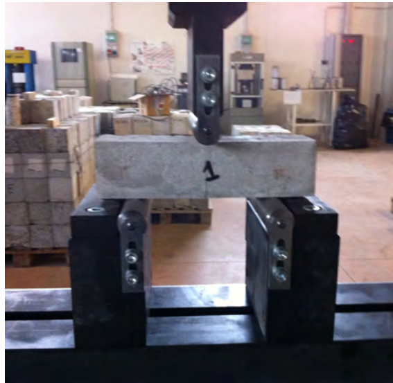
Figure 6 – Three-point bending test setup.
