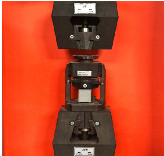
Figure 7 – Compression test setup.
