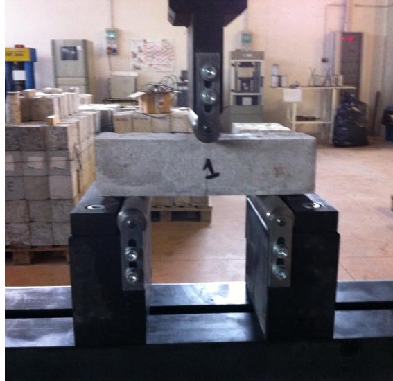
Figure 6 – Three-point bending test setup.
