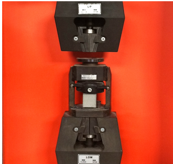
Figure 7 – Compression test setup.
