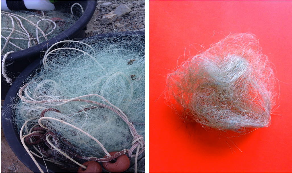
Figure 1 – Examined Nylon 6 waste fishing nets.
