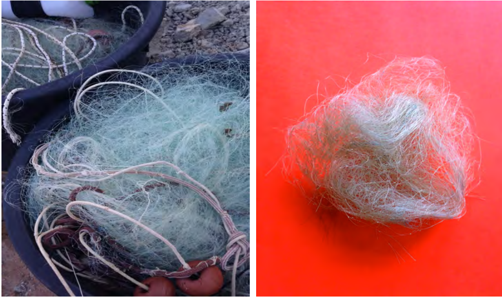
Figure 1 – Examined Nylon 6 waste fishing nets.
