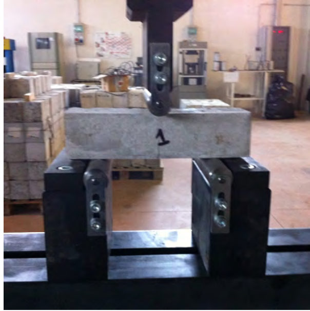
Figure 6 – Three-point bending test setup.
