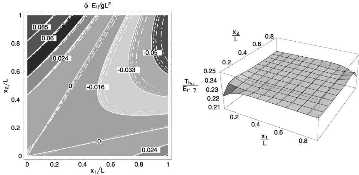
Fig. 10. Convergence of LSM solutions (SFF) for the Example 3 in the terms of the Airy function  $\varphi$  (left), and LSM distribution of the stress  $T_{12}$  for a  $10 \times 10$  mesh ( $h = 0.10L - 121$  DOF, right). (—) Example 1; (-----) Example 2; (.....) Example 3.
