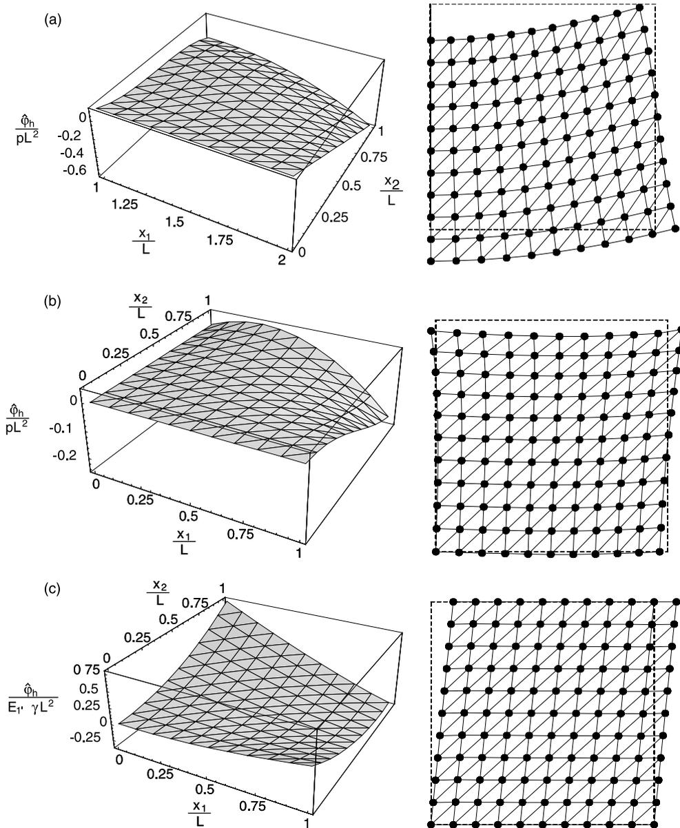
Fig. 7. (a)–(c) Polyhedral stress functions (*left*) and deformed shapes (*right*) given by the LSM (SFF) for the Examples 1 (*top*), 2 (*middle*), and 3 (*bottom*). (----)  $h = 0.25L$  (25 DOF); (---)  $h = 0.10L$  (121 DOF); (- - - - -)  $h = 0.05L$  (441 DOF); (—) exact solution.
