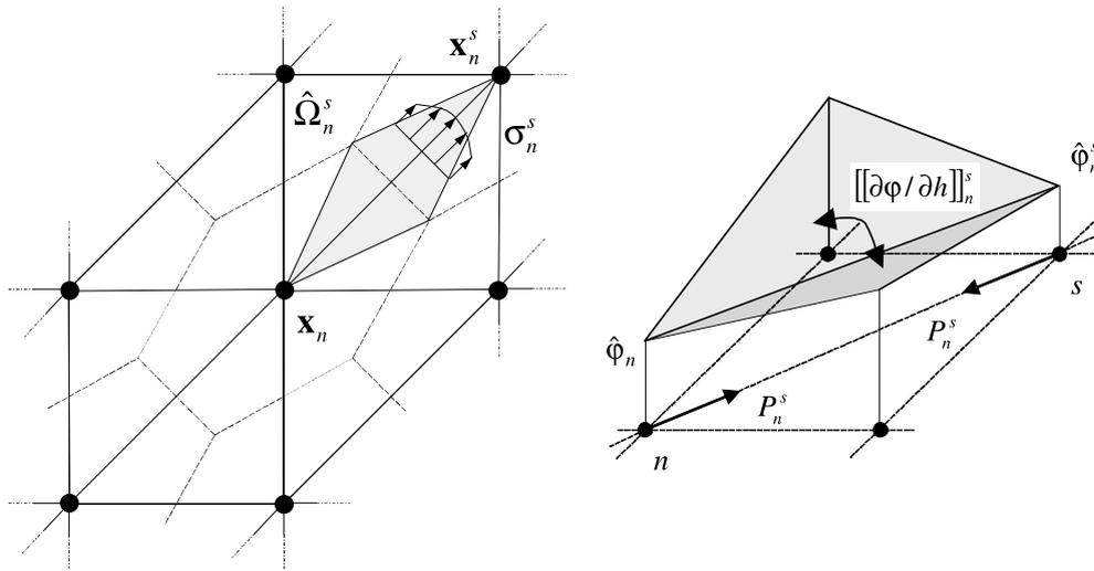
Fig. 5. Axial force  $P_n^s$  associated with a polyhedral stress function  $\hat{\varphi}$ .
