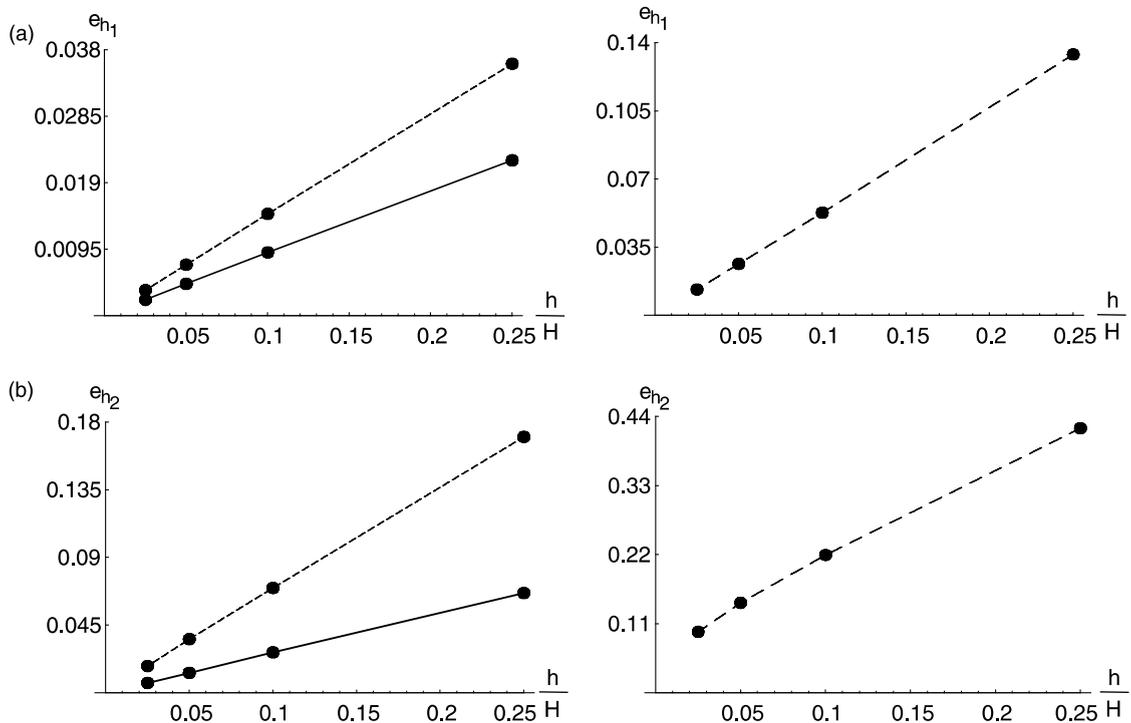
Fig. 11. (a) Plots of the LSM approximation error  $e_{h_1} = \|\hat{\varphi}_h - \varphi_0\|_1 / \|\varphi_0\|_{4,\infty}$  as a function of the mesh size. (—) Example 1; (-----) Example 2; (.....) Example 3. (b) Plots of the LSM approximation error  $e_{h_2} = \|\hat{\mathbf{T}}_h - \mathbf{T}_0\|_0 / \|\varphi_0\|_{4,\infty}$ .
