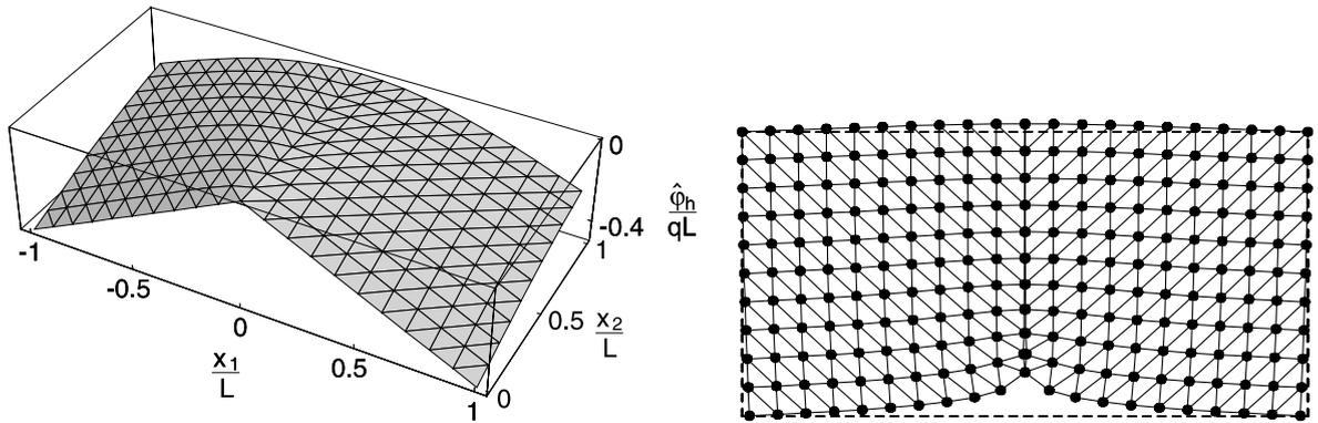
Fig. 13. Polyhedral stress function and deformed shape for the Flamant problem ( $h = 0.10L$ ). (---)  $h = 0.25L$ ; (----)  $h = 0.10L$ ; (-----)  $h = 0.05L$ ; (—) exact solution.
