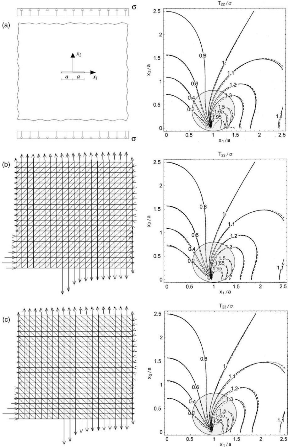
Fig. 16. (a)–(c) Stress concentration around a slit-like crack loaded in tension—Contours of the normal stress  $T_{22}/\sigma$  for a finite element solution ( $15 \times 15$  mesh, 450 DOF, top) and two LSM solutions (SFF, 441 DOF, middle and bottom).
