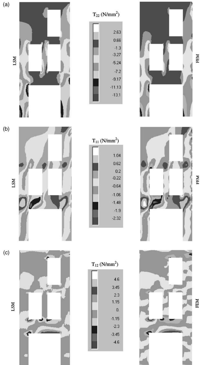
Fig. 20. (a) LSM (NDF) and FEM maps of the stress component  $T_{22}$  within the wall for an equal number of nodes. (b, c) LSM (NDF) and FEM maps of the stress components  $T_{11}$  and  $T_{12}$  within the wall for an equal number of nodes.
