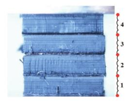
A multilayer structure of alternating layers of aligned carbon nanotubes and Cu foils. The mechanical behavior of this structure under compression can be modeled by a series of bistable springs.
