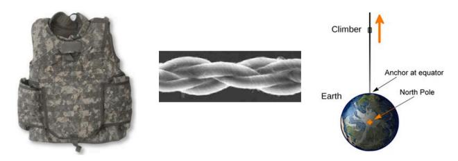
Due to their very high strength-to-weight ratio and excellent electrical and thermal properties, carbon nanotubes have been proposed for a variety of applications. This includes possible replacements for Kevlar protective vests (left) since carbon nanotubes can be spun into tough yarns (center); carbon nanotubes have even been proposed for the cable of a space elevator.
