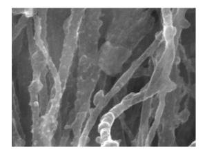
Carbon nanotube arrays can be customized both during and after synthesis. Pictured above are individual nanotubes (of approximately 50 nm diameter) which have been modified with MnO<sub>2</sub> particles on their surfaces. This modification could be useful both for increasing the compressive strength of the arrays and for electrochemical applications.
