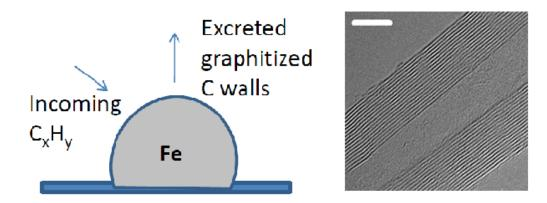
While there are a number of synthesis pathways to obtain carbon nanotubes, typical chemical vapor deposition techniques rely on transition metal catalysts such as Fe, which are observed to absorb carbon at high temperatures, and can excrete it in graphitic form (diagram on left); typical carbon nanotubes can consist of many concentric cylinders (right, 5 nm scale bar).
