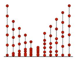
Axial strain localization in a mesoscopic chain of five bistable springs. The spring collapse mimics the local kinking of compressed carbon nanotubes.
