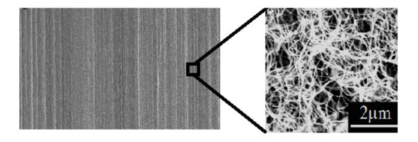
Carbon nanotube arrays can be synthesized which have foam-like characteristics and display a hierarchical structural arrangement. At the mesoscale, the material appears very ordered, with well-aligned carbon nanotube bundles (left); but if one looks at a smaller length scale, the individual carbon nanotubes are observed to be highly laterally entangled (right).
