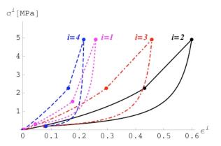
The regions corresponding to the various springs undergo nonuniform collapse. This behavior is captured by experimentally observing and mathematically modeling the separate stress-strain behavior for each region.
