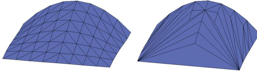
Fig. 2. (Left) Elastic solution in terms of the Airy stress function for a clamped masonry beam. (Right) Corresponding concave hull.
