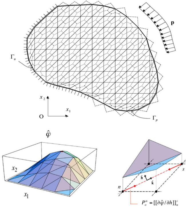
**Fig. 1.** (Top) Primary and secondary meshes of a plane body described through the lumped stress method. (Bottom) Polyhedral approximation of the Airy stress function and current lumped stress  $P_n^s$ .
