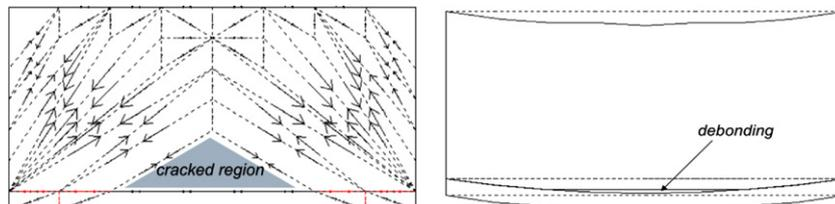
Fig. 4. LSDM solution for a clamped masonry beam strengthened with a steel profile at the bottom edge. (Left) Lumped stress network. (Right) Deformed shape.
