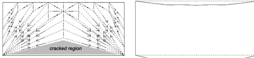
Fig. 3. LSDM solution for a clamped masonry beam. (Left) Lumped stress network. (Right) Deformed shape.
