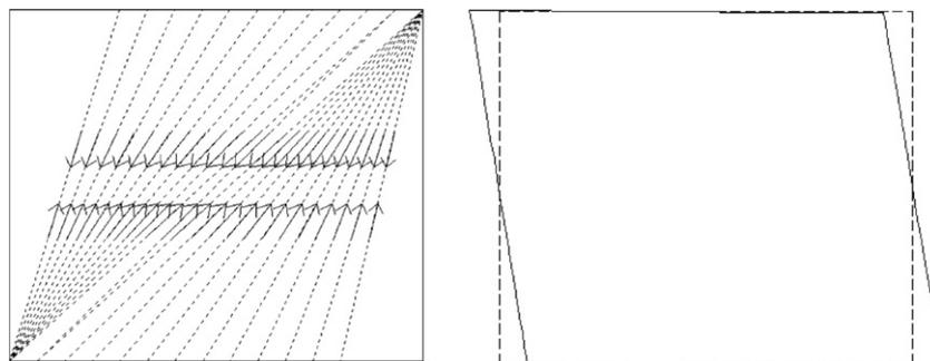
Fig. 5. LSDM solution for a shear wall. (Left) Lumped stress network. (Right) Deformed shape.
