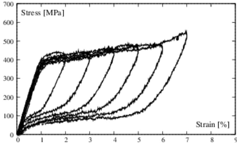
Figure 5: Stress-strain response of the NiTi wire sample to 7 consecutive tensile cycles.
