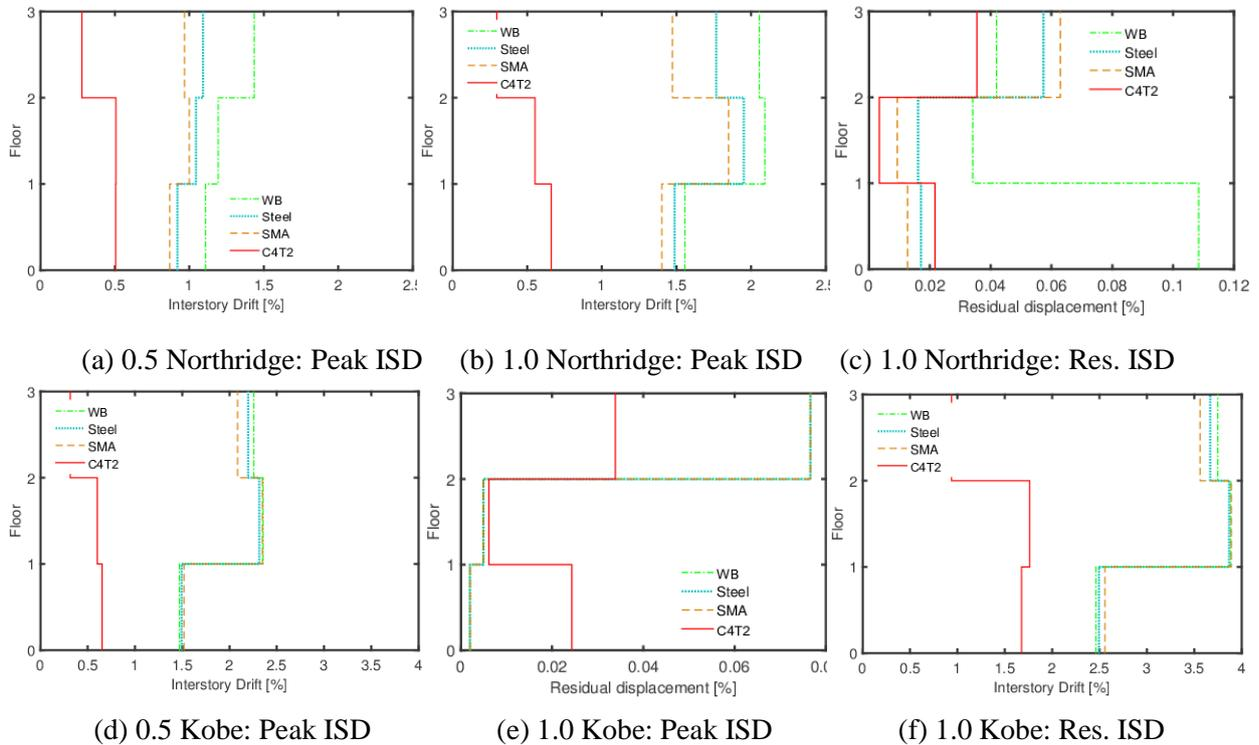
Figure 10: Peak and residual ISD along the height of the building.
