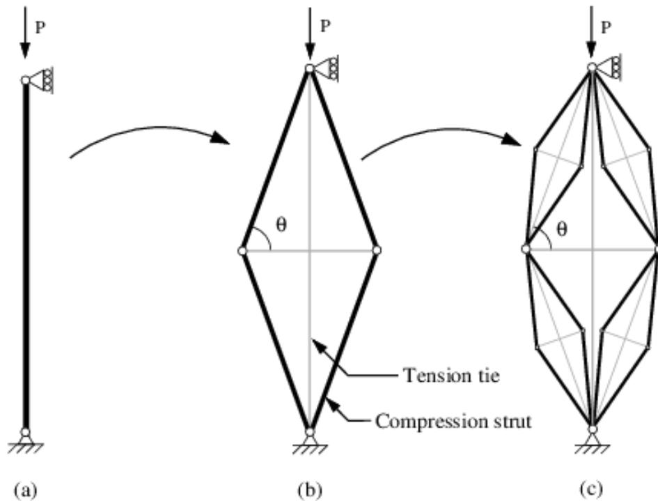
Figure 1: Proposed C4T2 tensegrity brace
