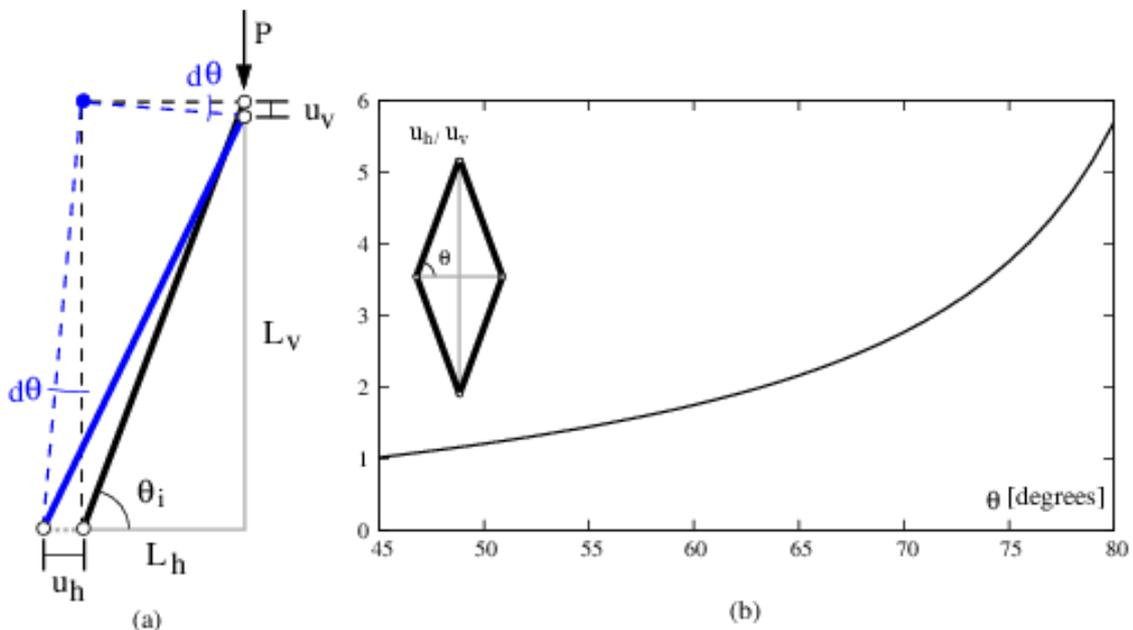
Figure 3: Displacement amplification factor of the C4T2 brace in the small displacement regime.
