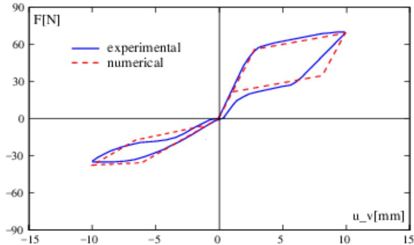
Figure 6: Comparison between numerical and experimental force-displacement diagrams.
