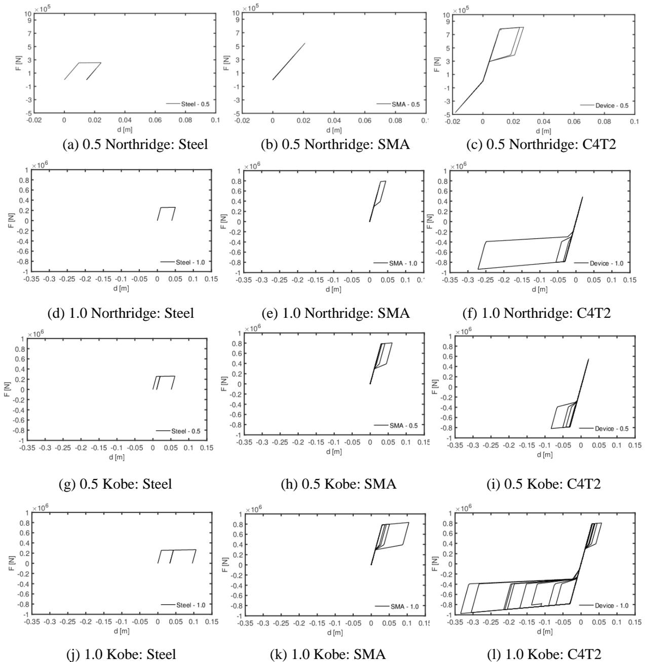
Figure 9: Force-displacement responses of the most stressed braces of the analyzed building models.
