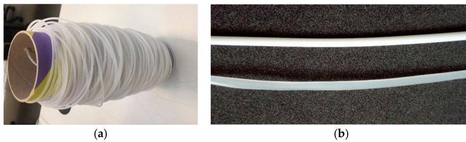
**Figure 1.** Pictures illustrating the AQ27000 filaments: (a) manufactured in the Aquafil plant of Arco (Trento, Italy) and a comparison between an AQ24000-T filament (b, top) and an AQ27000 filament (b, bottom).
