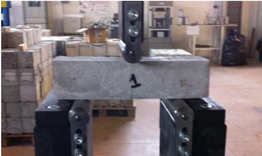
**Figure 5 – Three-point bending test setup.**
