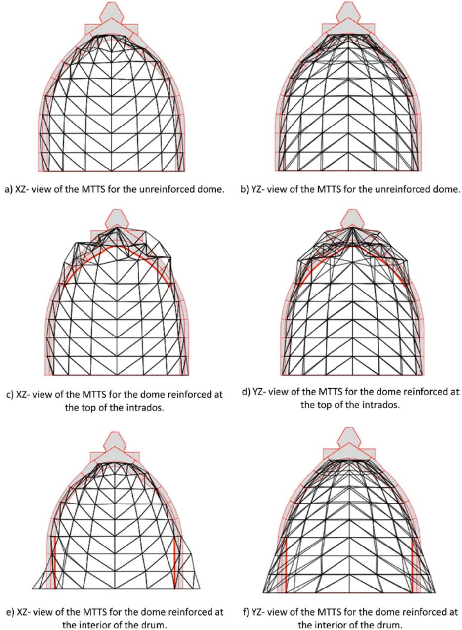
Figure 6: MTTs for seismic loading of the unreinforced and reinforced domes.
