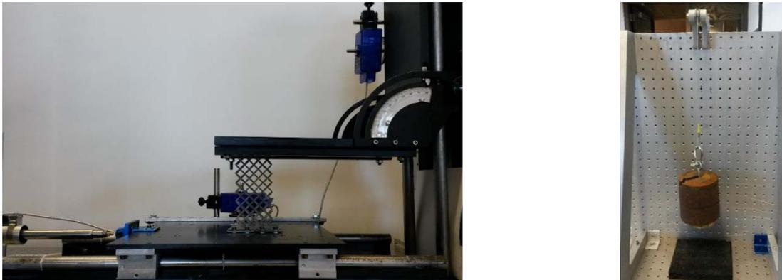
Figure 4. Left: overall view of the experimental setup. Right: counter balancing system introduced to remove platen self-weight.
