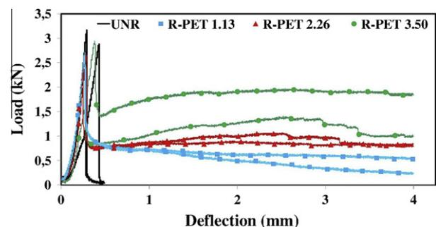
Fig. 2. Load-deflection curves of tested mortars at 7 days.
