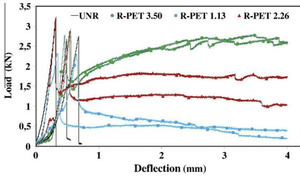
Fig. 3. Load-deflection curves of tested mortars at 28 days.
