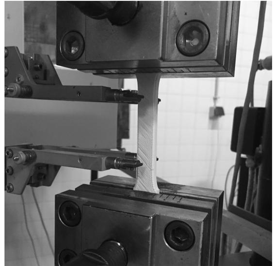
**Figure 6:** Tensile testing procedure.
