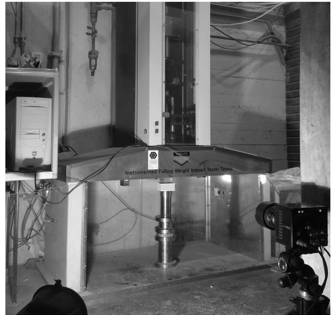
Figure 15: Rosand IFW5 instrumented falling weight impact tester.
